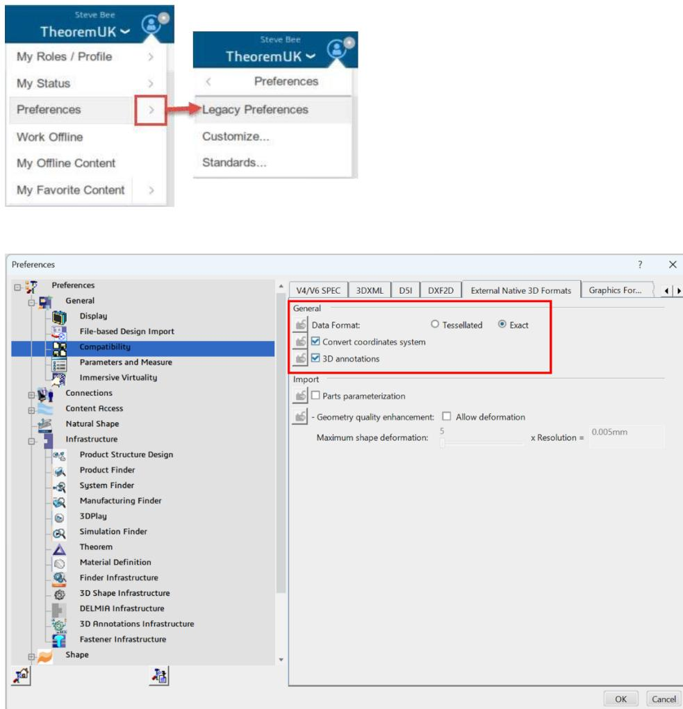
This page is a standard Dassault Page that enables the user to set the preferred mode of conversion (in this case Exact). It also enables the user to apply general options such as '**Convert coordinates system**' and '**3D annotations**'.
